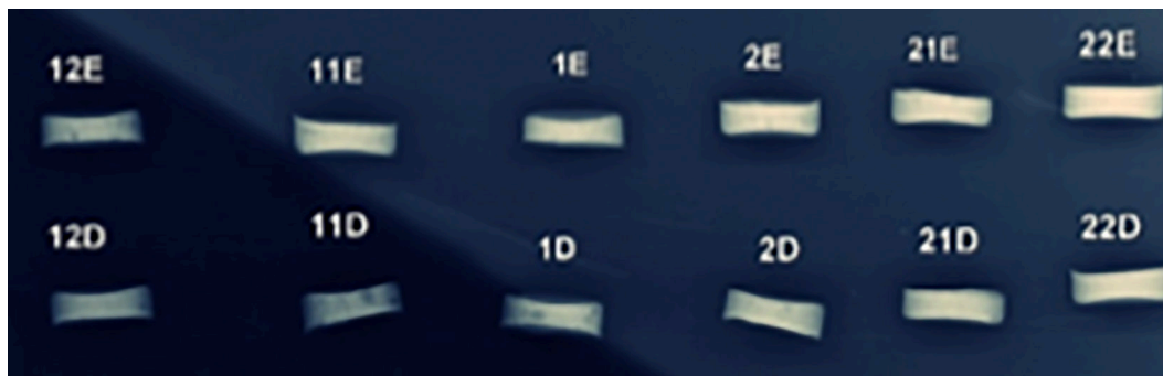
Figure 1. Conventional X-ray image of the composite material Silicon Rubber/PVA + \text{ZrO}_2 [1 % (11-12E/D), 3 % (1-2E/D), and 5 % (21-22E/D)].
