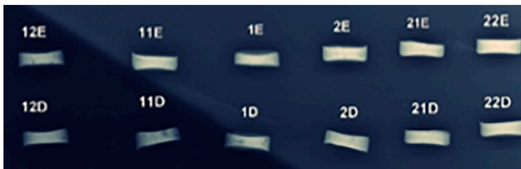
Figure 1. Conventional X-ray image of the composite material Silicon Rubber/PVA + \text{ZrO}_2 [1 % (11-12E/D), 3 % (1-2E/D), and 5 % (21-22E/D)].
