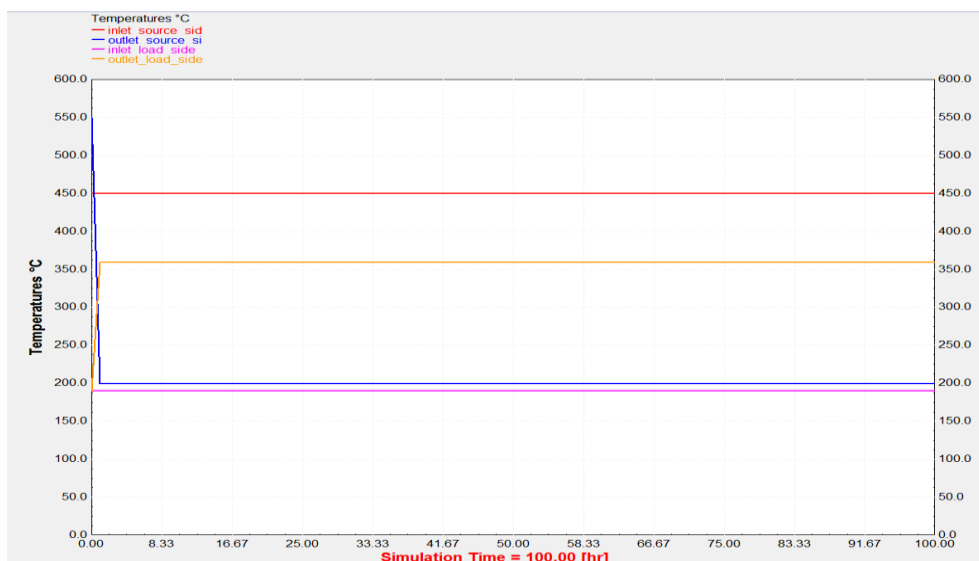
Figure 69. Inlet and outlet temperature in the source and load side in the power block generator.
