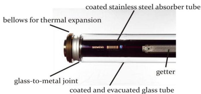
Figure 26. Receiver tube components (Source: Gunther et al., 2011 ).
