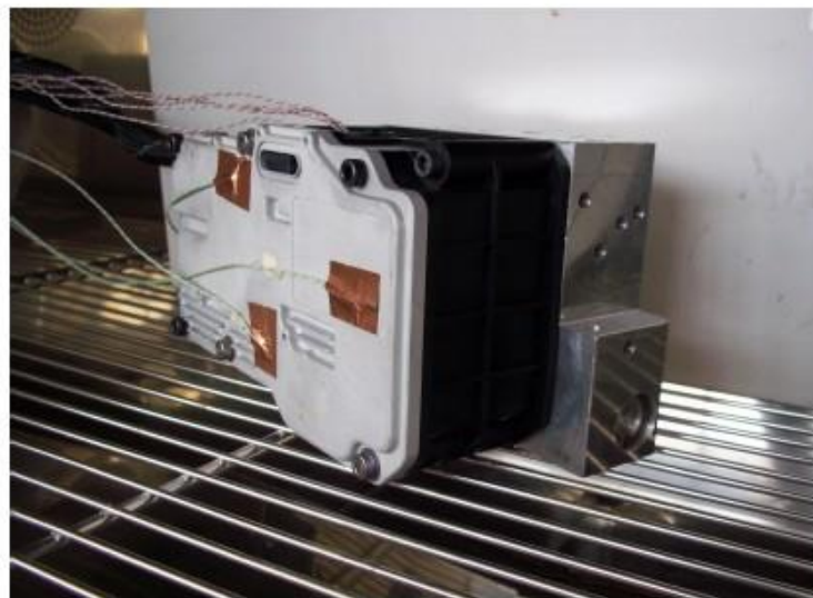
Picture 4: Heat Sink T/C positioning
