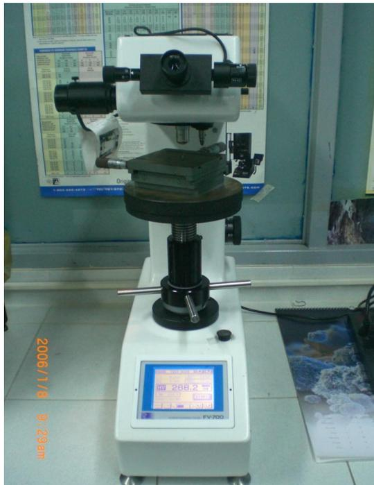
**Figura 2. 4.** Vickers Hardness Tester, Marca Buehler, Modelo FV-700
