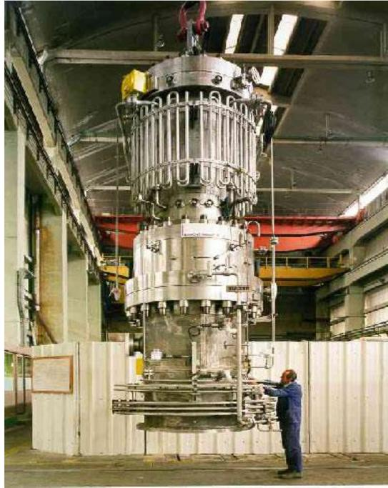
Figura 2.15. Bomba helicon-axial submarina.
