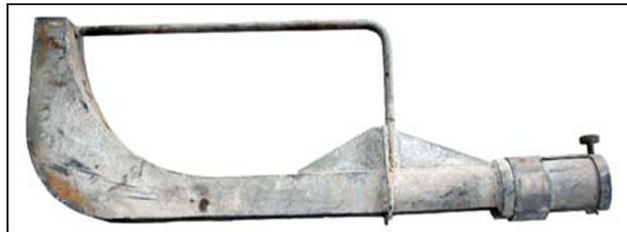
Fig. II.17: Goose Neck (tomado del TOP Operator Manual de SLB)
