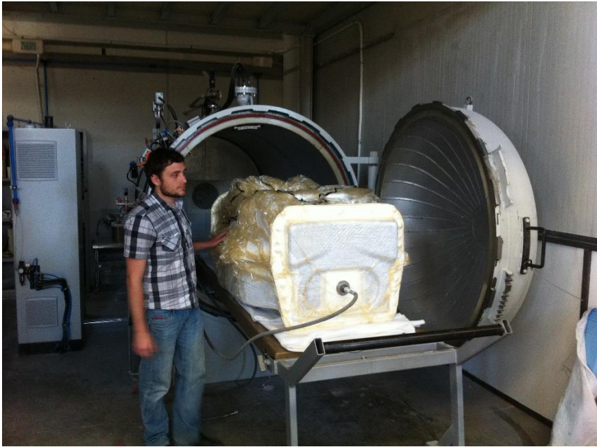
Laminated Inner skin with vacuum bag ready for the autoclave
