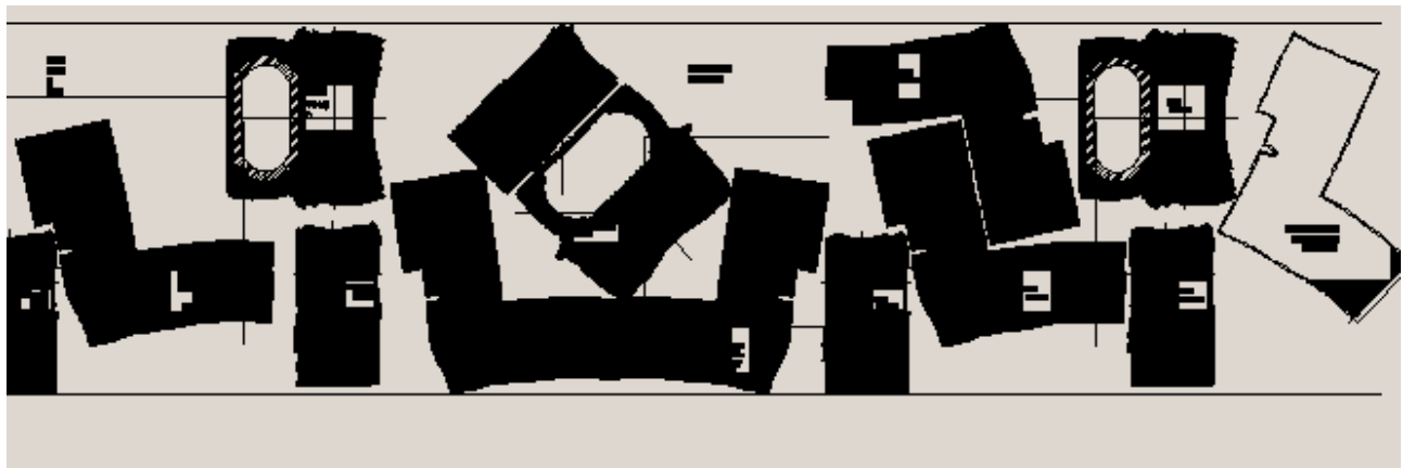
Figure 47- Section of the nested plies to be cutted
