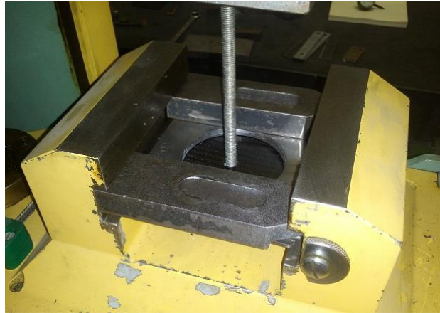
Figure 41- Pullout test of the safety harness attachments
