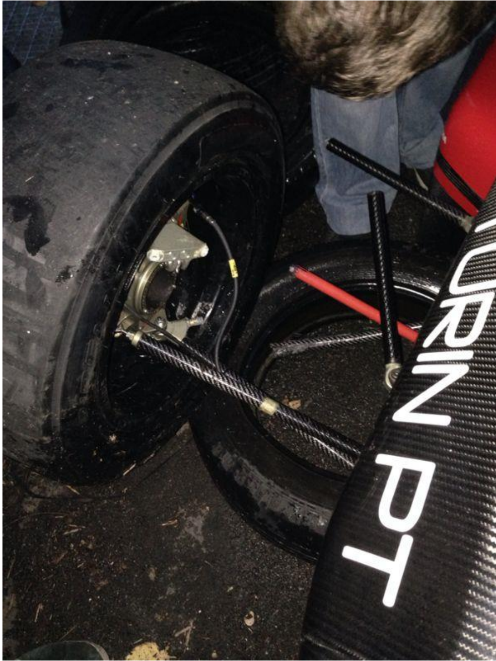
Figure 49- Suspension breakage during crash
