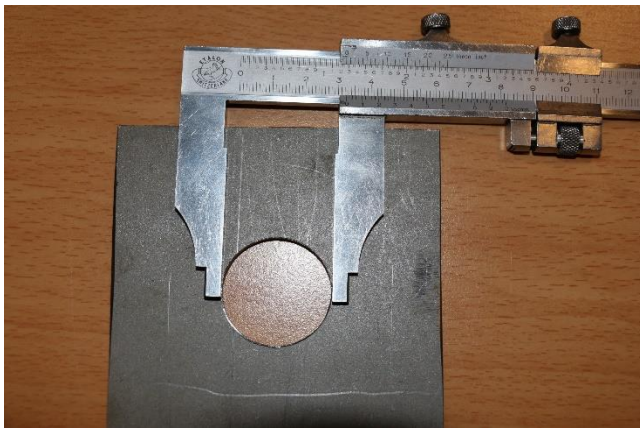
Figure 37 - Tooling details to perform the test. Support (left), Indentator (right)
