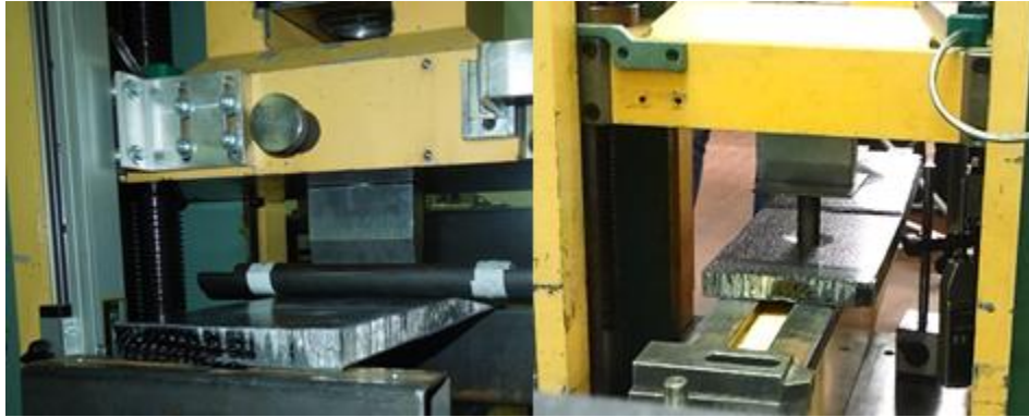
Figure 21 - (left) 3 Point Bending Test, (Right) Perimeter Shear Test
