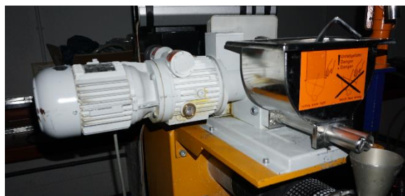
Figure 10. Twin screw doser for masterbatch.
