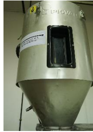
Figure 8. PIOVAN Hopper desiccant dryer for PLA and REX-PLA extrusion.
