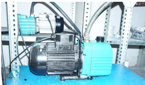
Figure 9. Vacuum pump used during extrusion.
