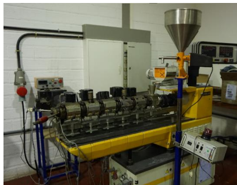
Figure 3. Co-rotating Twin Screw Extruder COLLIN Kneter 25 x 36D.
