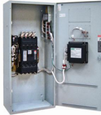
Fig. 4: Three pole Non-Automatic, electrically operated 400 ampere switch shown in Type 1 enclosure.
