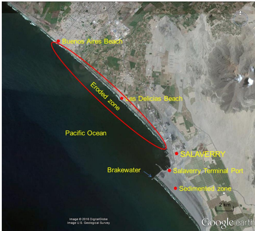
Figure 5. Satellite view of Salaverry Terminal Port, Peru, in January 2015, with about 600 meters of sand accumulation. Strong erosion is evident from the Las Delicias beach (Image from Google Earth).
