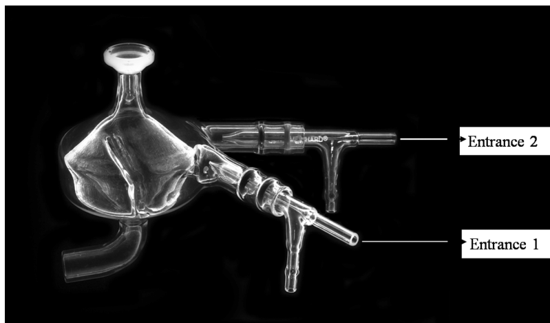
Figure 1. Schematic diagram of the modified cyclonic spray chamber with dual nebulization.
