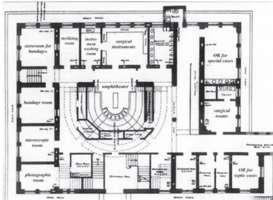
Arriba: Plano del pabellón quirúrgico William J Sims del hospital Roosevelt. (Tomado de Clemons B.J. The first modern operating room in America. AORN Journal 2000; 71:164-170.)
